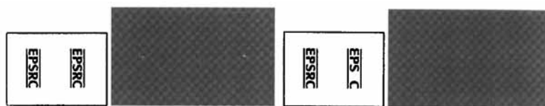
Figure 9. Input and output planes for the optical recogniser inspecting a label that matches and a label with defect.
