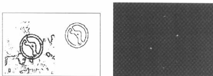
Figure 7. Testing the FBP-SLM correlator; Input image and output plane.
